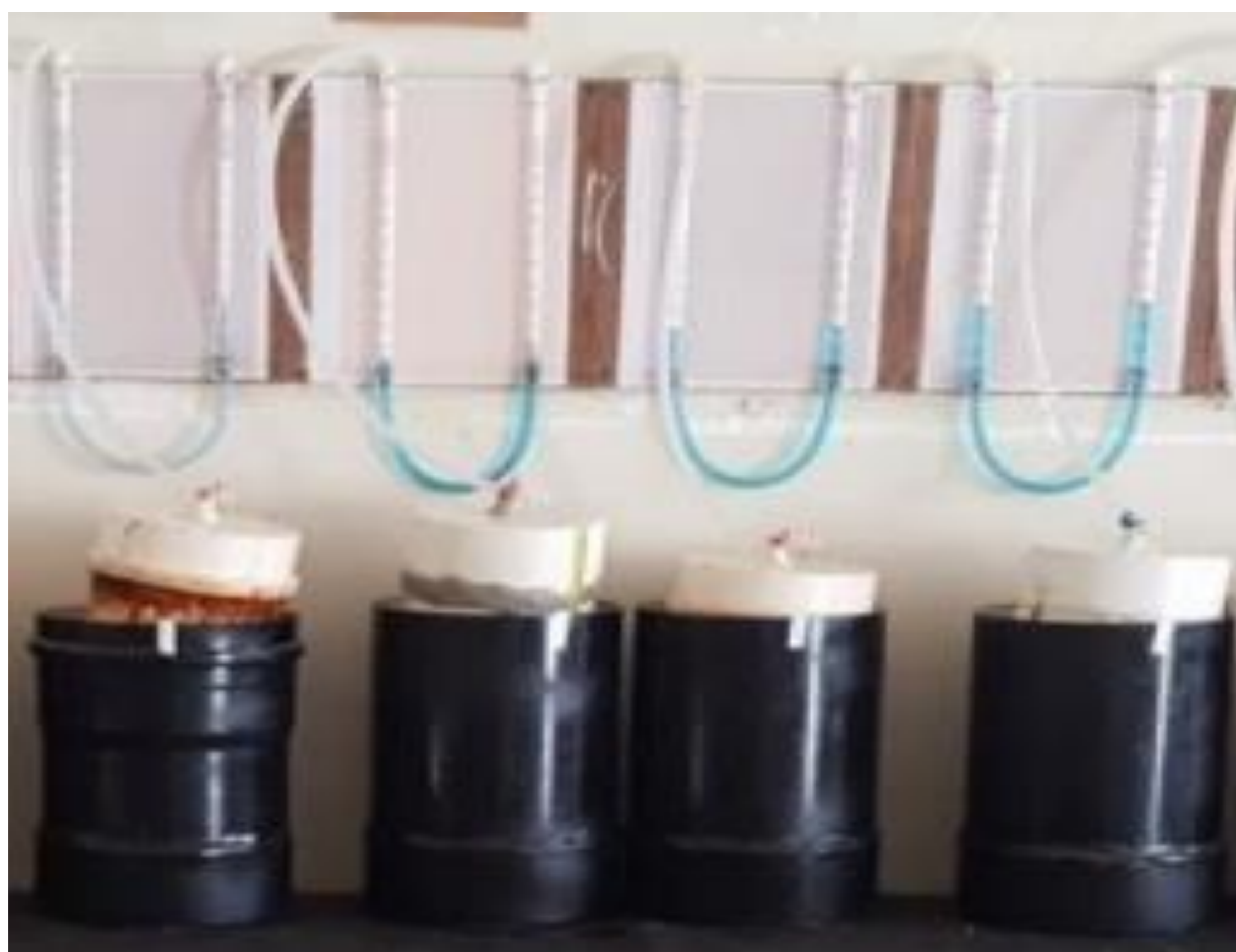
Figure 1. Indian model benchtop biodigesters
