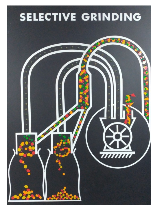
Figure 4. Schematics of selective grinding mode (material fractionation).
