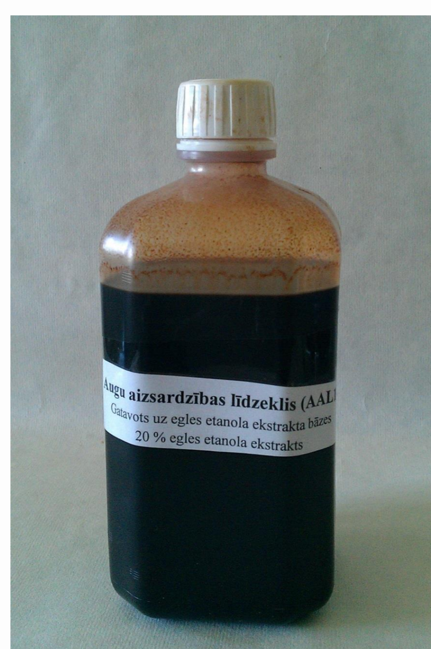
Fig.2. Spruce bark ethanol extract formulation used in test
