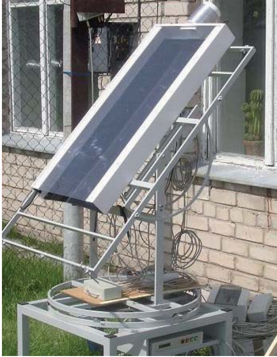
Fig. 1. Sun following collector with steel-thin plate absorber. Fig. 2. View of solar collector with steel-plate absorber.
