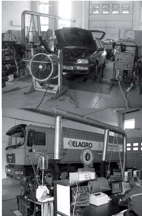
Fig. 1. Vehicles used in the experiments (VW Golf 1.9TDI and MAN 19,464).
